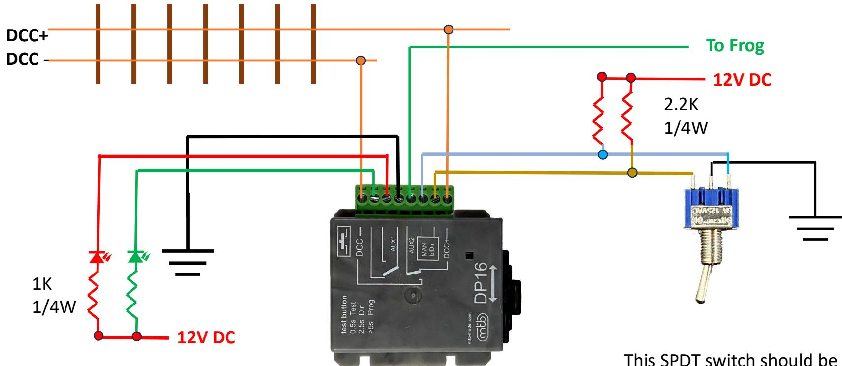
This SPDT switch should be Continuous unless being driven by a diode matrix
