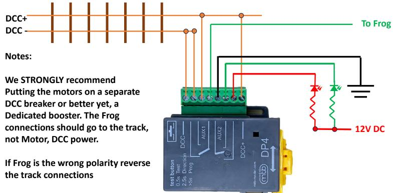
If the wrong LED is lighting reverse the connections to the LEDs
