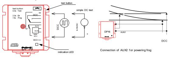
For manual control there are two bidirectional inputs MAN biDir, which are galvanically isolated from DCC signal. They can be used for manual operation.
